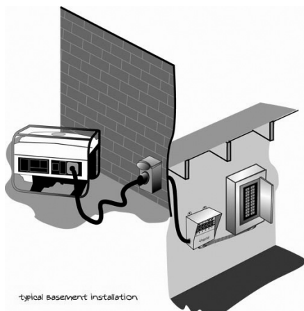
Generator Plugged into Outdoor Power Inlet Box Wired to Transfer Switch Next to Basement Load Center (POSSIBLE KIT INSTALLATION)
