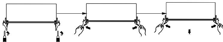
Figure 60 Removing a Module
