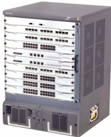
Figure 2 3Com Switch 8810 (10-Slot Chassis)
