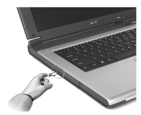
When the power is off, you can eject the drive tray using the emergency eject hole. See page 62.
