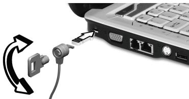
Wrap the computer security lock cable around an immovable object such as a table or handle of a locked drawer. Insert the lock into the notch and turn the key to secure the lock. Some keyless models are also available.
