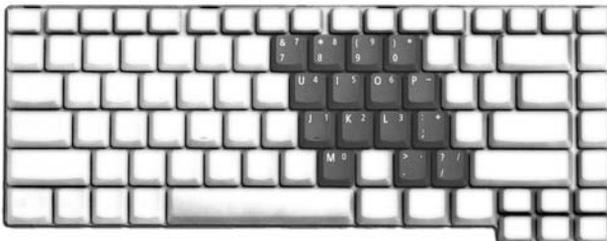
The embedded numeric keypad functions like a desktop numeric keypad. It is indicated by small characters located on the upper right corner of the keycaps.
