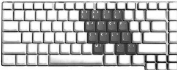
The embedded numeric keypad functions like a desktop numeric keypad. It is indicated by small characters located on the upper right corner of the keycaps.
