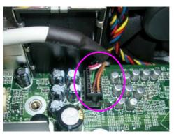
15.Remove the Front card reader cable and Front audio cable.
