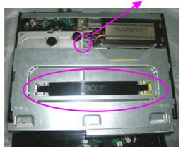
6. Detach ODD & HDD data and power cable.
