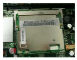
21.Remove the Wireless LAN Cable then release the LAN card.
