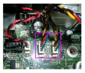
19.Release eight screws then remove the System FAN.
