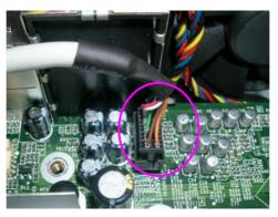
**5**. Remove the Front card reader cable and Front audio cable.
