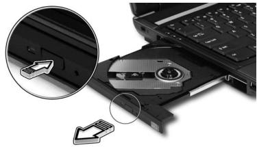
Insert a paper clip to the emergency eject hole to eject the optical drive tray when the computer is off.
