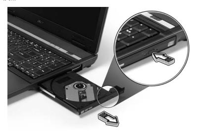
Insert a paper clip to the emergency eject hole to eject the optical drive tray when the computer is off.
