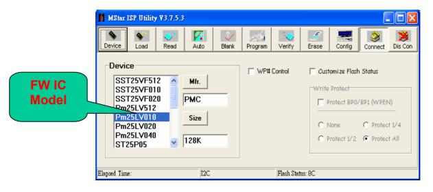
Secondly, download FW software: first select "READ", and then load FW software in Rooter (Fig.2).
