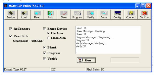
Note: if programming fails or success rate is not high, click "Config" and adjust its speed in "E2PROM DEVICE SETTING"
