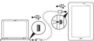
Using the micro USB to USB cable, connect the micro end into your tablet and the other end into your computer.
