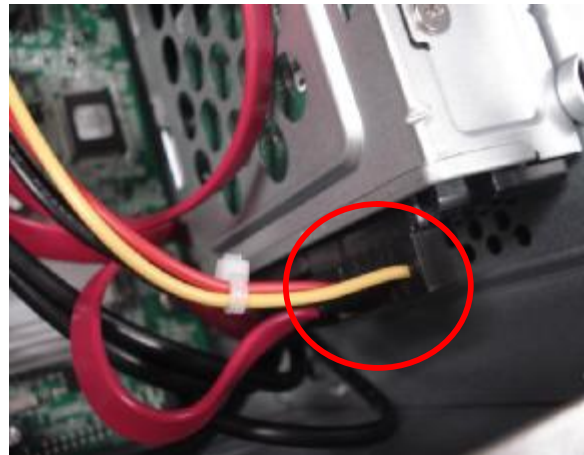
Insert the HDD power-cable
