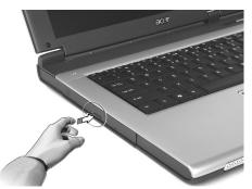
When the power is off, you can eject the drive tray using the emergency eject hole.
