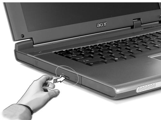
When the power is off, you can eject the drive tray using the emergency eject hole. See page 56.
