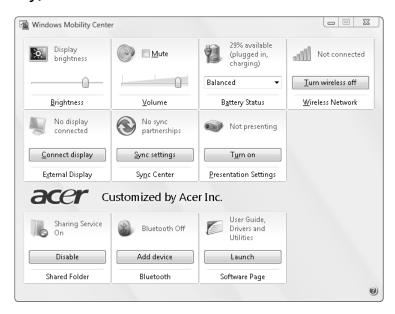
The Windows Mobility Center collects key mobile-related system settings in one easy-to-find place, so you can quickly configure your Acer system to fit the situation as you change locations, networks or activities. Settings include display brightness, power plan, volume, wireless networking on/off, external display settings, display orientation and synchronization status.
