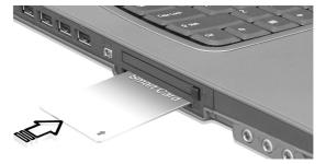
To remove the Smart Card first press the Smart Card (a) and remove the Smart Card (b) as shown in the illustration below.
