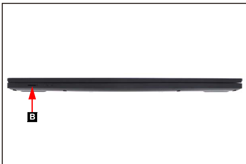
Figure 1-2. microSD Card Removal
