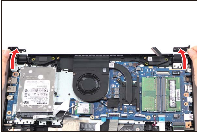
Figure 1-22. LCD Module Removal
