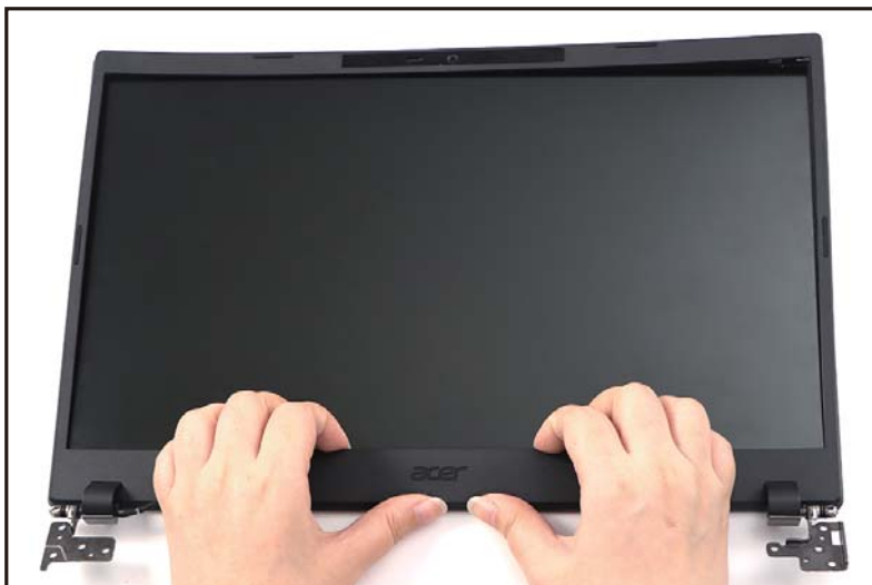
Figure 1-44. LCD Bezel Removal
