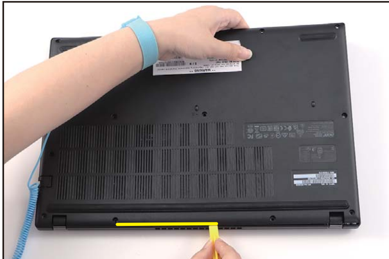
Figure 1-5. Base Cover Removal
