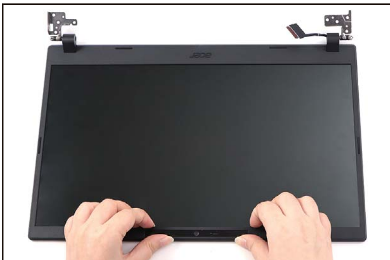
Figure 1-41. LCD Bezel Removal
