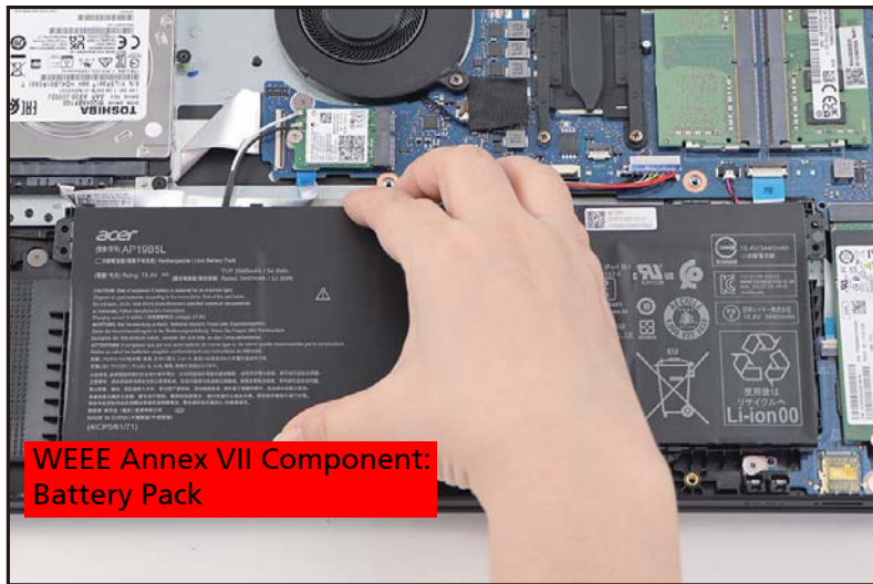
Figure 1-8. Battery Pack Removal
