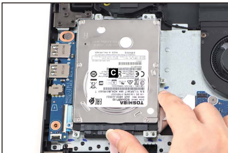
Figure 1-27. HDD Module Removal
