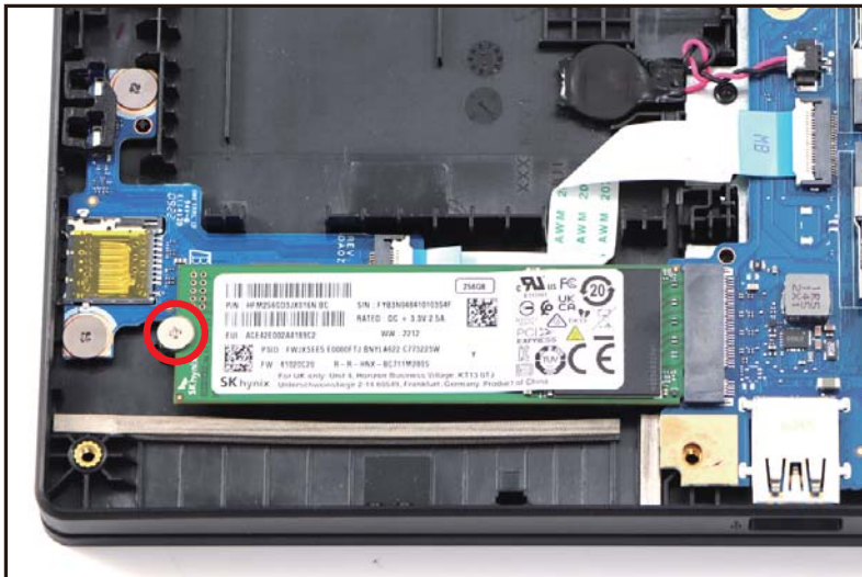
Figure 1-24. SSD Module Removal
