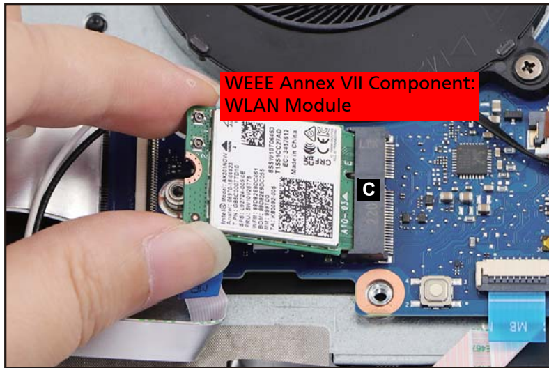
Figure 1-16. WLAN Module Removal
