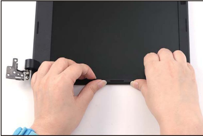
Figure 1-42. LCD Bezel Removal
