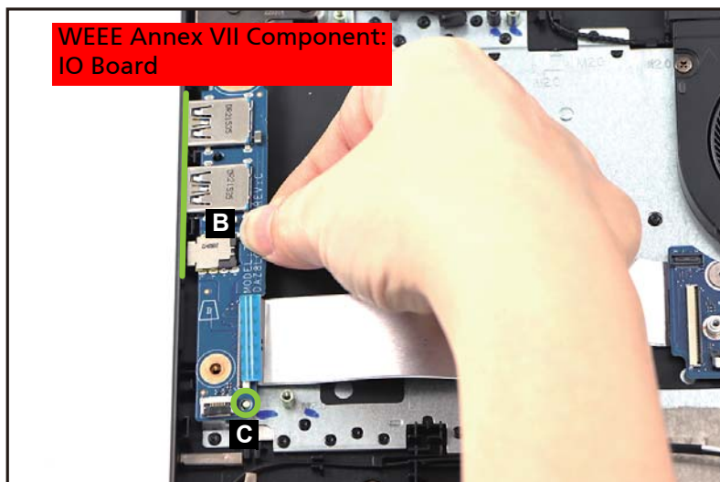
Figure 1-39. IO Board Removal
