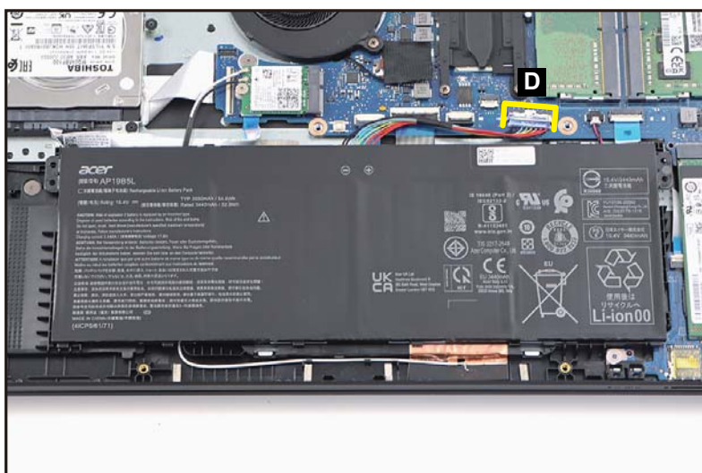
Figure 1-7. Battery Pack Removal
