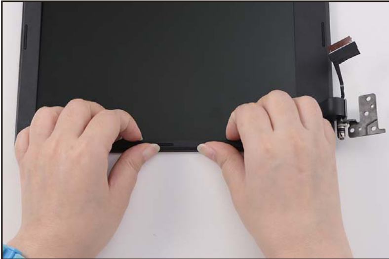
Figure 1-43. LCD Bezel Removal
