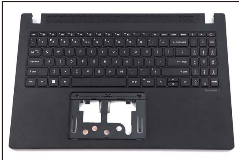
Figure 1-50. Top Assembly (Keyboard)
