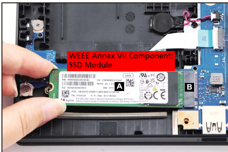
Figure 1-25. SSD Module Removal
