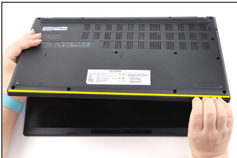
Figure 1-4. Base Cover Removal
