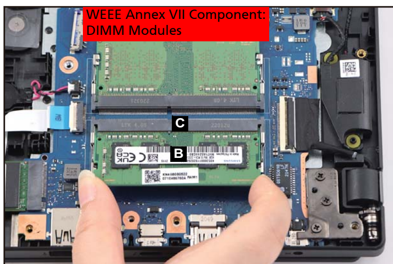
Figure 1-18. DIMM Modules Removal
