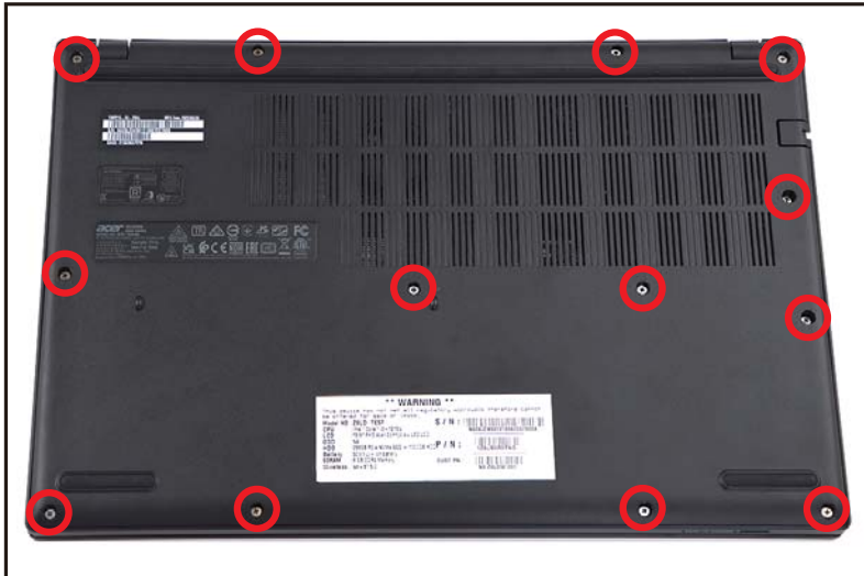
Figure 1-3. Base Cover Removal
