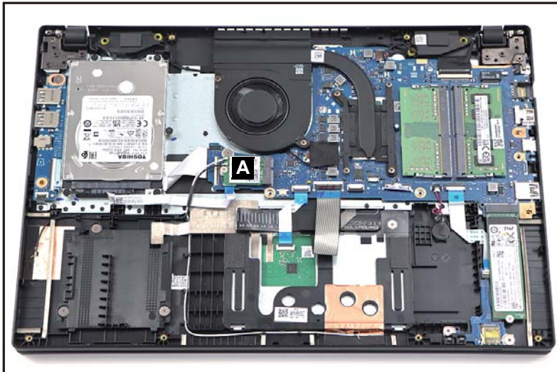
Figure 1-14. WLAN Module Location
