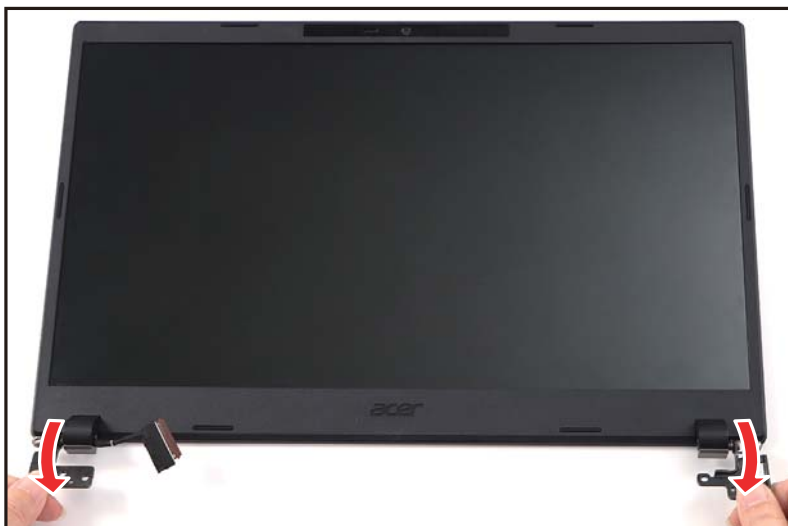
Figure 1-40. LCD Bezel Removal
