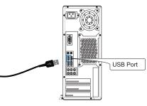
8. When your computer recognizes scanner, return to the orignal window
