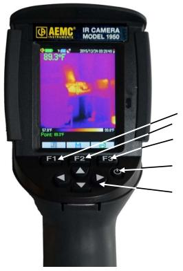
Multiple-function keys associated with the display on screen
