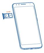
**Step 3.** Position the SIM card or Micro SD card in the tray correctly, aligning the cutout tab and gently snap into place. Be sure the edges are aligned.
