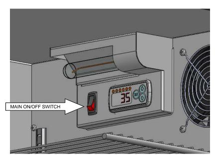
Switch the unit ON using the main ON/OFF power switch, located inside the cabinet, below the light. Immediately after the unit is switched on, the cabinet light and inside evaporator fans will start operating. Check the temperature setting which has been set at the factory to 35°F.
