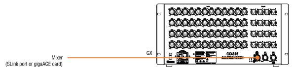
Switch on the mixer first, then the GX Expander. The GX port Lnk/Err indicators flash at a steady rate when the link is established. The red error indicator lights if a communication error is detected.
