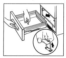
Then, with drawer out about halfway, pull metal clip located in center of drawer bottom upward as far as it will go (about 2 inches). The drawer can now be pulled all the way out of the compartment.
