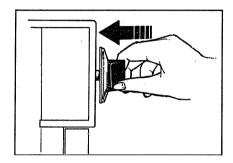
Push the control knob in and turn it to LITE. On electric ignition models, you will hear a little clicking noise—the sound of the electric ignition spark that lights the burner.
