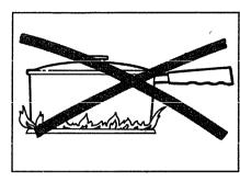
NEVER LET THE FLAME EXTEND UP THE SIDES OF THE COOKWARE. Any flame larger than the bottom of the cookware is wasted and only serves to heat the handles.
