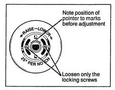
Note to which mark the pointer is pointing. To make an adjustment, carefully loosen (approximately one turn), but do not completely remove the two screws that hold the skirt to the knob. Hold the knob blade in one hand and the outer skirt in the other hand.
