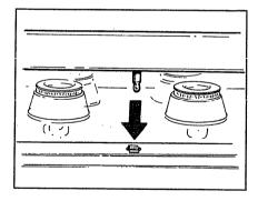
To replace the cooktop if you have removed it, insert the two tabs at the back of the cooktop into slots at the base of the backguard. Lower cooktop into place, applying pressure until tab on underside snaps into catch at top front center of range.
