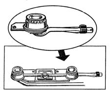
Note: A screw holds each of the burners in place to keep them from wobbling around during shipment. Remove and discard the shipping screw. Tilt the burner to one side at the end closest to the ignitor and move it toward the back of the range. This disengages it from the gas valve at the front of the range, and it lifts out easily.
