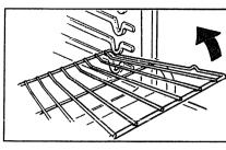
The shelves are designed with stoplocks so when placed correctly on the shelf supports, they will stop before coming completely out of the oven and will not tilt when you are removing food from them or placing food on them.
