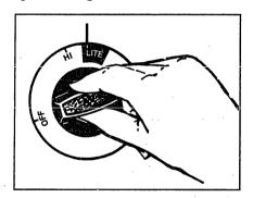
After the burner ignites, turn the knob to adjust the flame size.
