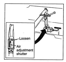
To adjust the flow of air, loosen the Phillips head screw and rotate the shutter to allow more or less air into the burner tube as needed.
