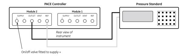
**Note:** Module 2 reference port open to atmosphere or to reference port of the pressure standard.
