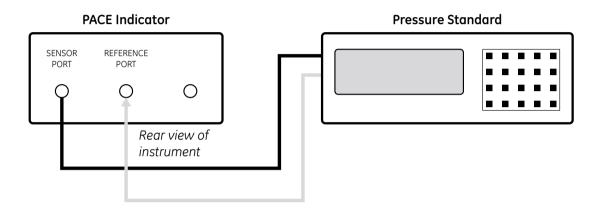
**Note:** Indicator reference port open to atmosphere or to reference port of the pressure standard.
