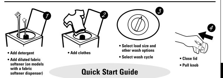
*NOTE*: When making a selection with any knob, simply point the knob anywhere within the shaded range for that setting.
