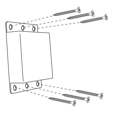
The GefenTV Extender for HDMI over one CAT5 should be mounted vertically on a wall or inside / outside a cabinet with wood / drywall screws as shown in the diagram above. There should be an inch or two of clearance between the edges of the unit and any walls or vertical surfaces to allow for enough clearance for connection and disconnection of the HDMI cable.
