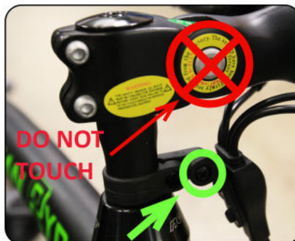
Fig. 1.6 Tighten Cable Screw (green)
