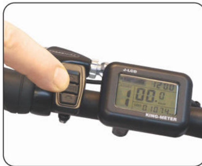
Fig. 9.2 Hold Down “MODE” Button for 2 Seconds
