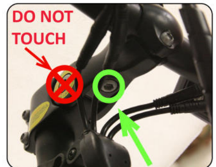
Fig. 1.7 Adjust Handlebar Angle (green)
