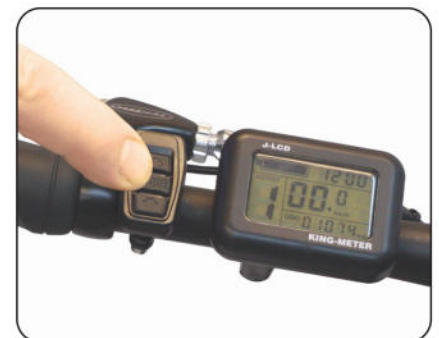
Fig. 10.2 Hold down “MODE” Button for 2 Seconds
