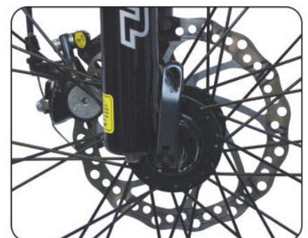
Fig. 2.5 Quick Release Lever In Closed Position
