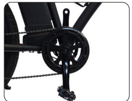
Fig. 3.2 Crank Arm, Right Pedal Inserted
