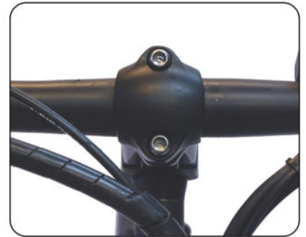
Fig. 1.4. Handlebar Faceplate With Tightened Bolts
