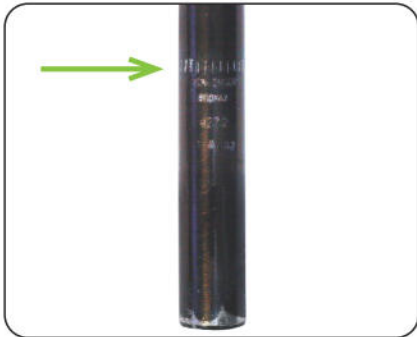
Fig. 4.1 Seat Post, “Minimum Insert Line”
