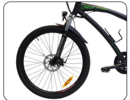
Fig. 2.7 Forks Secured Onto Front Wheel
