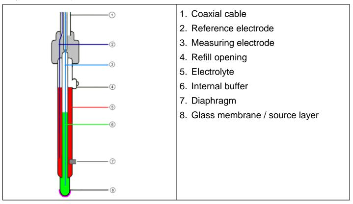
The diaphragm, which establishes a connection between the electrolyte and the liquid to be measured, can be designed in different ways. Clogging or soiling of the diaphragm is a frequent cause of a malfunctioning or sluggish electrode.
