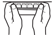
Hand-tighten sink flange
