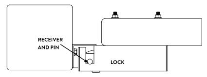
View looking down showing receiver pin lines up with gate lock
