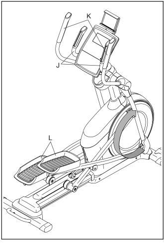
To dismount the elliptical, wait until the pedals (L) come to a complete stop. Note: The elliptical does not have a free wheel; the pedals will continue to move until the flywheel stops. When the pedals are stationary, step off the higher pedal first. Then, step off the lower pedal.
