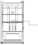
The air duct of temperature sensor part in wind tunnel cover of the fridge compartment
