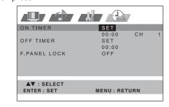
2 Press is or it to enter the hours and minutes at which you want your TV to automatically switch on.
