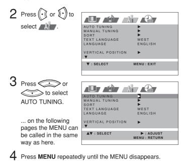
If no buttons are pressed for more than approx. 60 seconds, the MENU disappears automatically.
