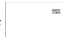
When the displayed time runs out, the unit will switch to standby. The display will disappear after approx. 4 seconds.
