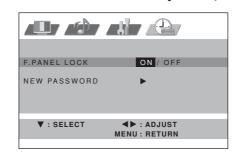
4 Press **MENU** repeatedly until the MENU disappears. If a button on the front panel is pressed, the message "F.PANEL LOCK" appears for approx 4 seconds.
