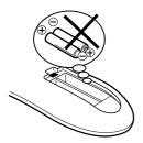
If the batteries have not been installed according to their polarities.
