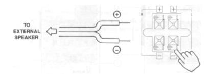
**CAUTION:** Do not connect Speakers simultaneously to the REAR SPEAKER terminal of the Projection TV and Amplifier. This could damage both the Projection TV and the Speakers. Your Hitachi TV was designed to use 8 speakers only. Any other type may
