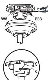
Receiver (B) correctly positioned in the mounting bracket.
