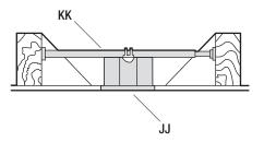
To hang your fan where there is an existing fixture but no ceiling joist, you may need an installation hanger bar (KK) (not included) as shown above.
