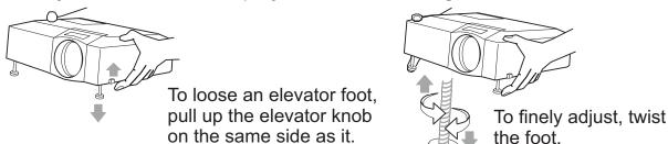
**△CAUTION** ► Do not handle the elevator knobs without holding the projector, since the projector may drop down.
