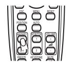
2. Use the ▲/▼ cursor buttons to adjust the zoom level. To move the zoom area, press the POSITION button in the MAGNIFY mode, then use the ▲/▼/◄/▶ cursor buttons to move the area. And to finalize the zoom area, press the POSITION button again.
