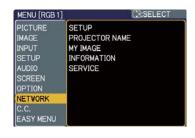
Select an item using the  $\blacktriangle/\blacktriangledown$  cursor buttons on the projector or remote control, and press the  $\blacktriangleright$  cursor button on the projector or remote control, or **ENTER** button on the remote control to execute the item. Then perform it according to the following table.
