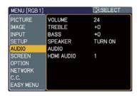
**NOTE** • If the volume is too loud or the treble or bass are overly emphasized, the case may vibrate or the sound may become distorted. Reduce the volume, treble or bass to eliminate the distortion.
