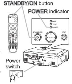
The projection lamp will light up and the **POWER** indicator will begin blinking in green. When the power is completely on, the indicator will stop blinking and light in steady green.
