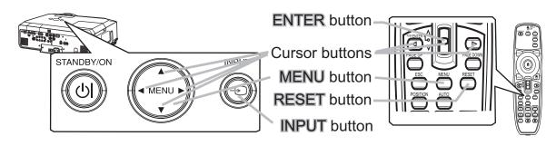
Press the MENU button on the remote control or one of the cursor buttons on the projector. The Advanced MENU, or EASY MENU that has priority just after powered on, will appear. If you want to move the menu position, use the cursor buttons after pressing the POSITION button. While the projector is displaying any menu, the MENU button on the projector works as the cursor buttons.
