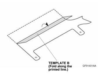
Raise the quarter window sunshade. Line up template B with the quarter window sunshade and switch trim on the left rear side trim panel as shown. Tape template B to the left rear side trim panel with masking tape.
