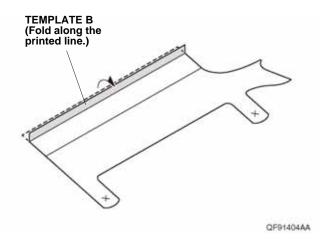
Line up template B with the quarter window and the switch trim on the left rear side trim panel as shown.
