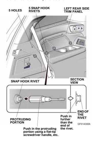
14. Place the left cargo liner on the left rear side trim panel as shown. Secure the left cargo liner to the left rear side trim panel with five snaps.
