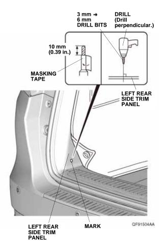
21. Install one snap hook rivet into the hole on the left rear side trim panel as shown.
