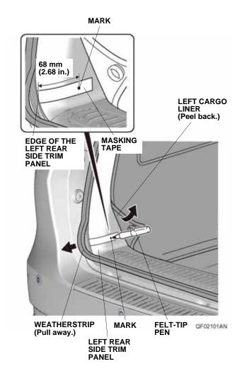
17. Attach a piece of masking tape to the left rear side trim panel as shown. Using a felt-tip pen, mark the masking tape as shown.
