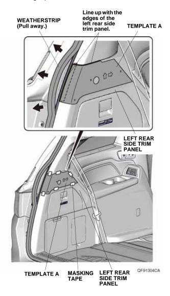
4. Using a pushpin, pierce the left rear side trim panel through template A at the locations shown. Remove template A.
