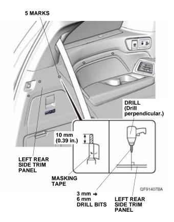
13. Install the five snap hook rivets into the five holes on the left rear side trim panel as shown.
