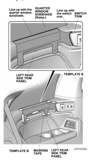
7. Using a pushpin, pierce the left rear side trim panel through template B at the locations shown. Remove template B. Go to step 11.
