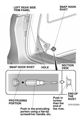
22. Secure the left cargo liner to the left rear side trim panel with one snap as shown.
