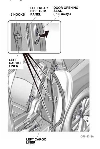
16. Pull away the weatherstrip, and peel back the left cargo liner. Attach a piece of masking tape to the left rear side trim panel just above the curve as shown. Using a felt-tip pen, mark the masking tape as shown.
