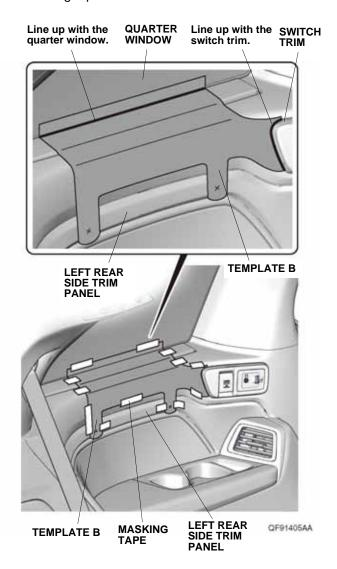
10. Using a pushpin, pierce the left rear side trim panel through template B at the locations shown. Remove template B.
