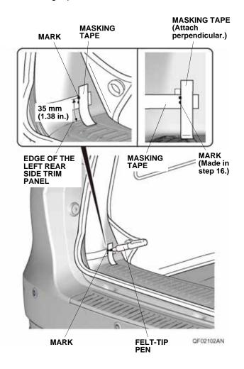
18. Using a pushpin, pierce the left rear side trim panel at the mark made in step 17 on the masking tape. NOTE: There are two marks on the masking tape. Before piercing the left rear side trim panel, verify you have the correct location. Make sure to pierce the mark perpendicular to the left rear side trim panel.
