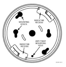
3. Secure the sensor to the mounting base by aligning the sensor's index tabs to the index tab recesses on the mounting base. While pushing in, turn the sensor clockwise until it locks. DO NOT touch the metal
