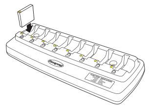
It is important that batteries are inserted into the charging pocket correctly. Inserting the battery incorrectly could result in damage to the battery or the charger. Do not "slam" or slide the battery into the pocket. This could damage the charger.
