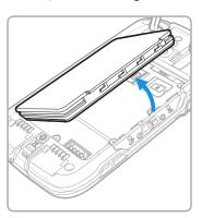
7. Lift up the edge of the SD card access door.
