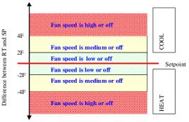
Fan speed ramping control algorithm
