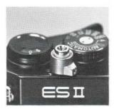
Your ES II is provided with a shutter lock. To prevent accidental shutter release, lock the shutter release button by moving the lock lever to the left. An "L" becomes visible.
