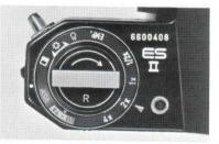
Use this control only when necessary to give intentional over- or under-exposures within the range of these factors while working on "AUTOMATIC". For example, set the dial at 2x or 4x when shooting against the light, and at 1/2x against dark backgrounds. In addition, the dial can be set between the indicated positions to achieve more specific exposure control.
