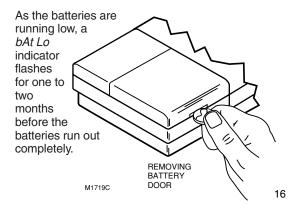
Replace the batteries as soon as possible after the indicator starts flashing.
