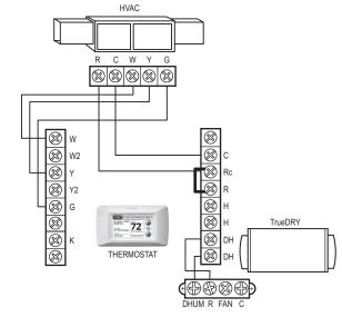
NOTE: THERMOSTAT MUST BE CONFIGURED TO DRIVE FURNACE FAN DURING DEHUMIDIFICATION CALL.
