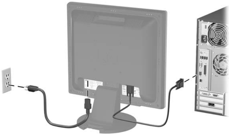
Connecting the Signal and Power Cables
