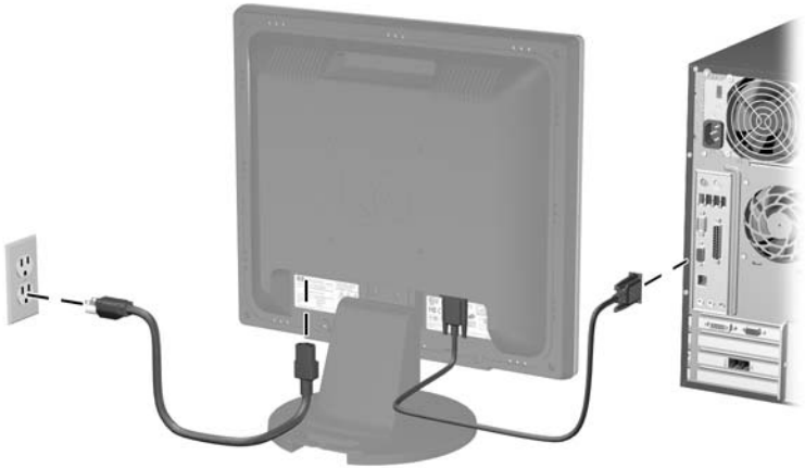
Connecting the Signal and Power Cables
