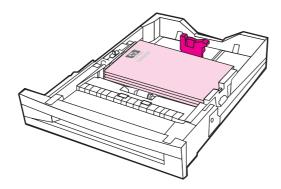
16. Insert Tray 2 into the printer. Make sure all trays are completely closed.
