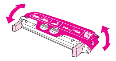
7. Remove the orange mylar strip and the orange shipping lock from the new print cartridge. Discard the lock.
