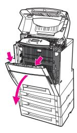
10. Grasp the green handles on the transfer unit and pull down.
