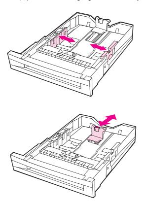
3. Load media face-up, making sure that the stack height of the paper does not exceed the maximum stack height mark in the tray.
