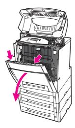
3. Grasp the green handles on the transfer unit and pull down.
