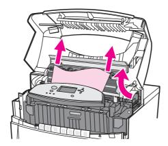
6. Inspect the fuser and remove any paper that is crumpled in the fuser.
