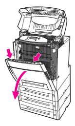
3. Grasp the green handles on the transfer unit and pull down.
