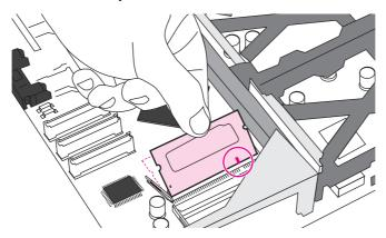
9. Push down on the DIMM until both latches engage the DIMM.
