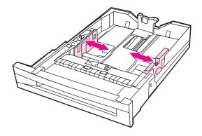
4. Load media face-up, making sure that the stack height of the paper does not exceed the maximum stack height mark in the tray.
