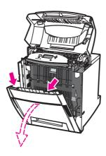
3. Grasp the green handles on the transfer unit and pull down.
