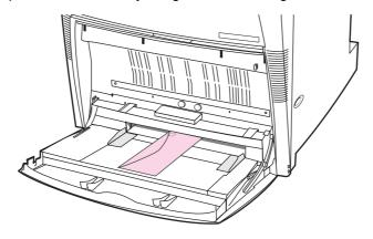
3. Adjust the guides to touch the envelope stack without bending the envelopes. Make sure the envelopes fit under the tabs on the guides.
