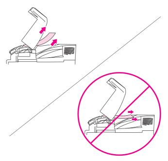
4. Open the fuser cover and pull up to remove any paper that is crumpled in the fuser.
