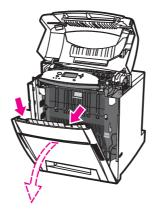
3. Grasp the green handles on the transfer unit and pull down.
