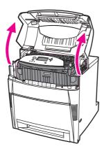
2. Firmly pull forward on the two green levers to disengage the fuser rollers.
