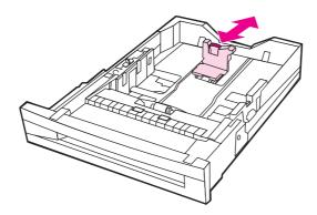
3. Adjust the paper width guide by squeezing the guide adjustment latch and sliding the guide to the width of the media being used.
