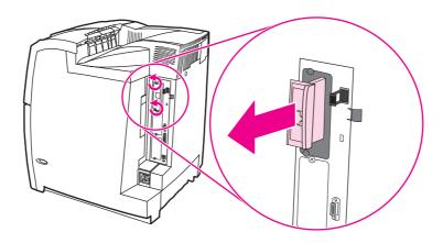
4. Firmly insert the HP Jetdirect print server card into the EIO slot. Insert and tighten the retaining screws that came with the print server card.
