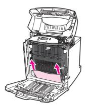
5. If the paper cannot be accessed from this location, grasp the green handles on the transfer unit and pull down.
