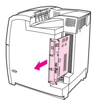
6. To replace a DDR DIMM that is currently installed, spread the latches apart on each side of the DIMM slot, lift the DDR DIMM up at an angle, and pull it out.
