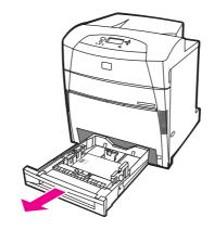
2. Slide the paper width and length guides all the way out.
