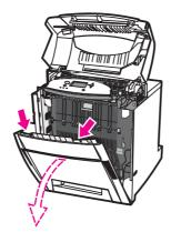
6. Grasp the green handles on the transfer unit and pull down.
