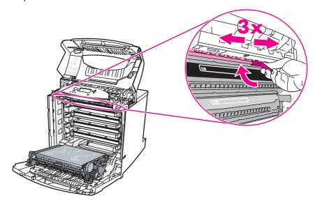
6. Close the ETB and store the cleaning brush inside the front cover. If you are replacing the ETB, a new cleaning brush is included.
