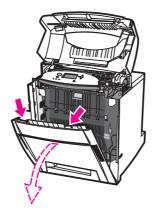
3. Remove the cleaning brush from inside the front cover.
