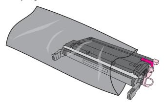
6. Grasp both sides of the cartridge and distribute the toner by gently rocking the cartridge from side to side.
