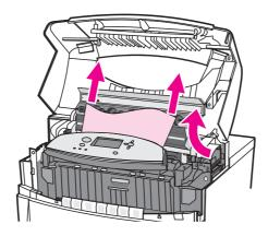
8. Inspect the fuser and remove any paper that is crumpled in the fuser.
