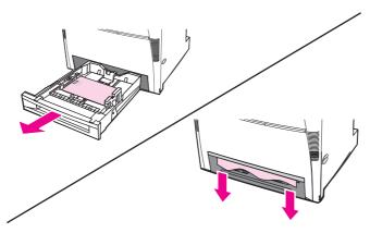
8. Inspect the paper path above to ensure that it is clear. To remove any partially fed paper, grasp the paper by both corners and pull down.
