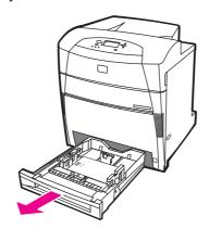
2. Slide the paper width and length guides all the way out.
