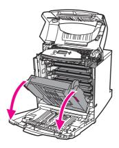
4. Remove the cyan print cartridge from the printer.
