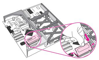
7. Remove the new DIMM from the antistatic package. Locate the alignment notch on the bottom edge of the DIMM.
