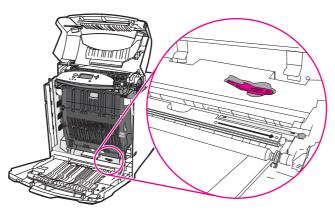
6. Insert the brush into the base notch and brush from right to left four or five times.
