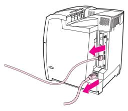
3. Locate the formatter board in the rear of the printer.
