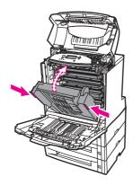
14. If you could not reach the paper with the transfer unit open in Step 12, grasp the paper by both corners and pull up.
