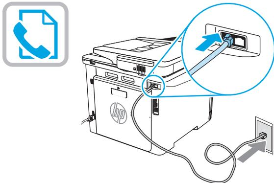
EN The printer uses an analog fax device. HP recommends using the printer on a dedicated analog telephone line.
