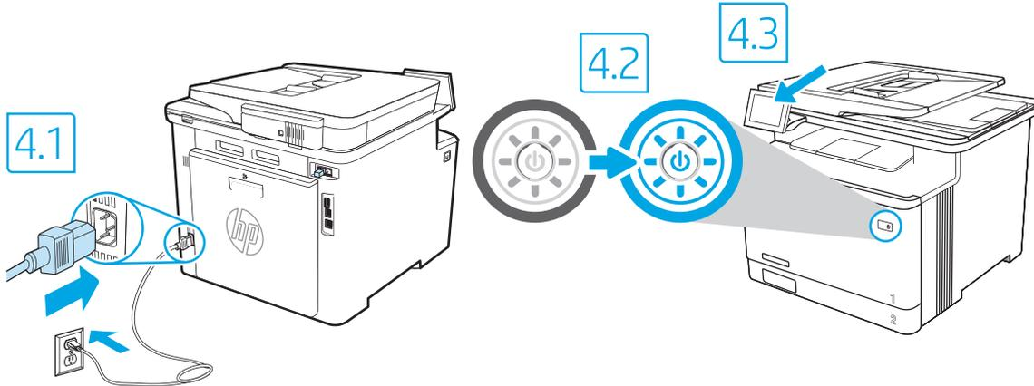
EN **4.1** Connect the power cable between the printer and a grounded AC outlet. **4.2** Turn on the printer. **4.3** On the **Initial Setup** screen, set the language, the location, the date/time format, and other features.
