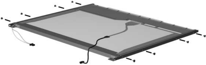
Removing the Display Panel Frame Screws
