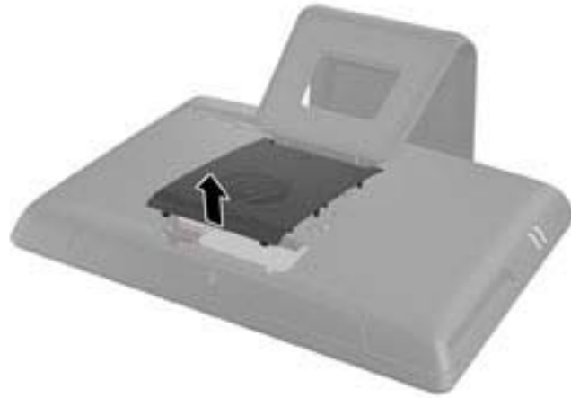
Figure 6-2 Removing the hinge cover panel
