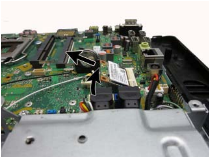
Figure 6-56 Removing the WLAN module
