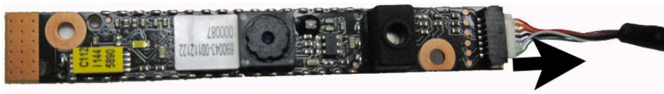
Figure 6-40 Disconnecting the webcam module
