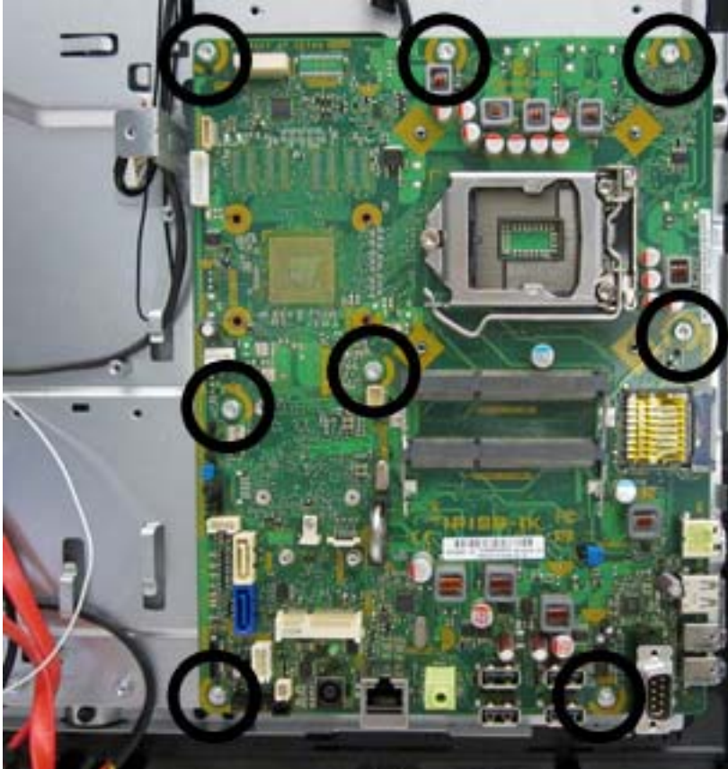
Figure 6-63 System board screw locations
