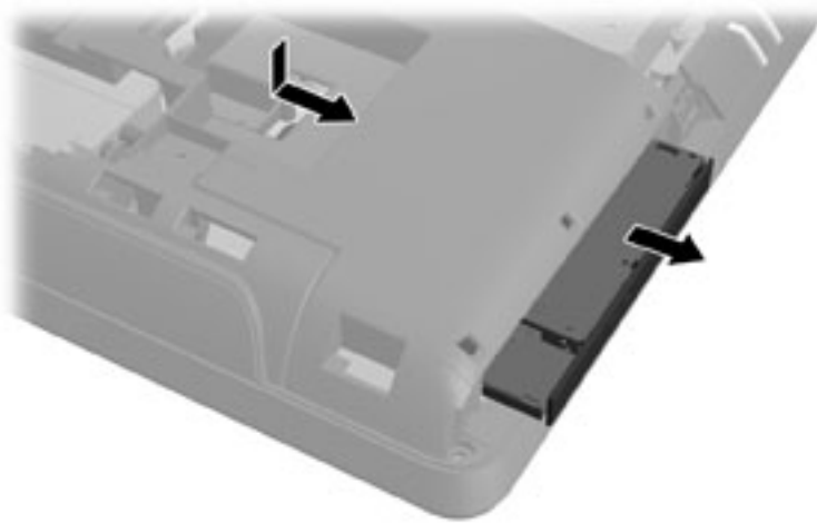
Figure 6-11 Removing the optical disc drive
