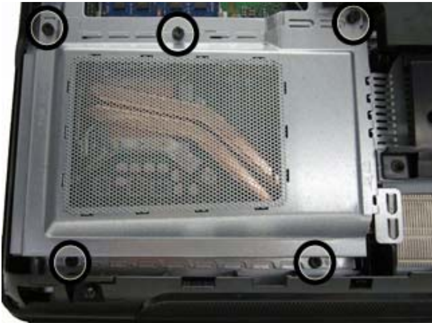
Figure 6-29 Heat sink cover screws
