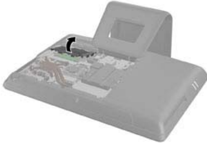
Figure 6-19 Removing the memory cover
