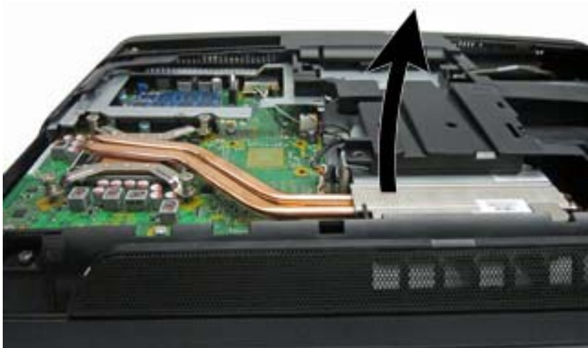
Figure 6-34 Removing the heat sink
