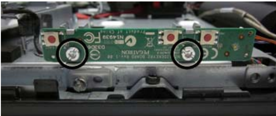
Figure 6-50 Sidekey board screws
