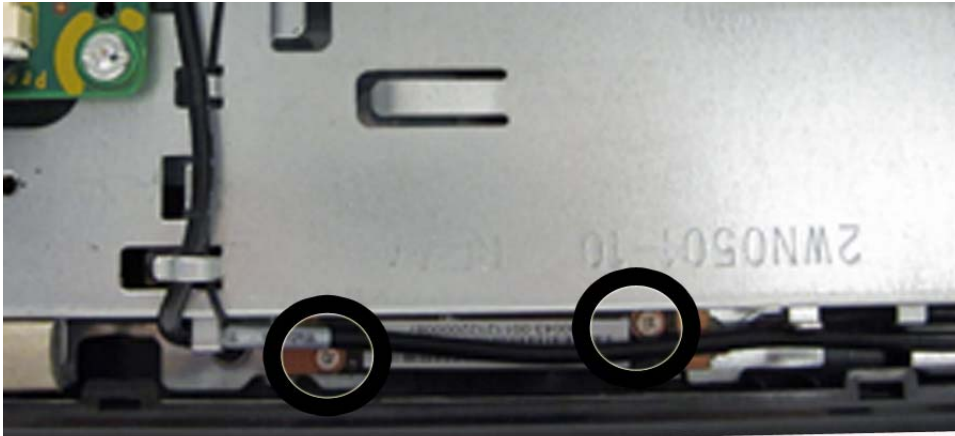
Figure 6-39 Webcam module screws
