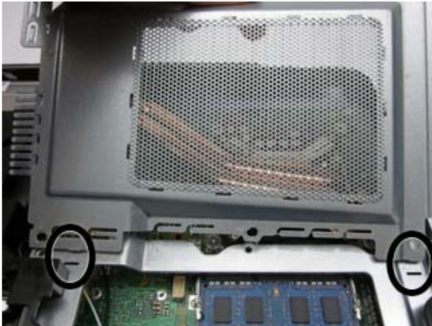
Figure 6-31 installing the heat sink cover
