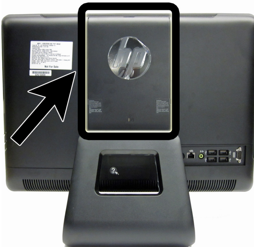
Figure 6-1 Hinge cover panel location
