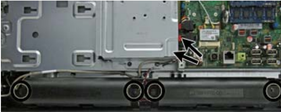
Figure 6-58 Removing the speakers
