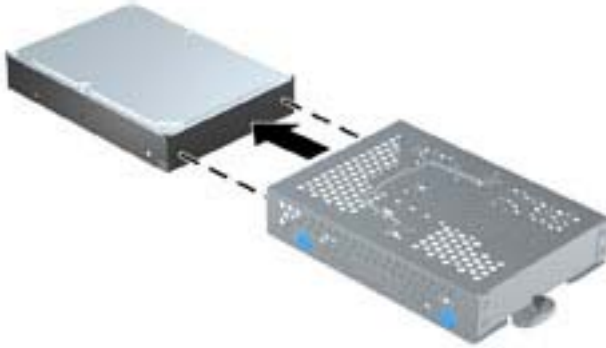
Figure 6-17 Removing the hard drive from the cage
