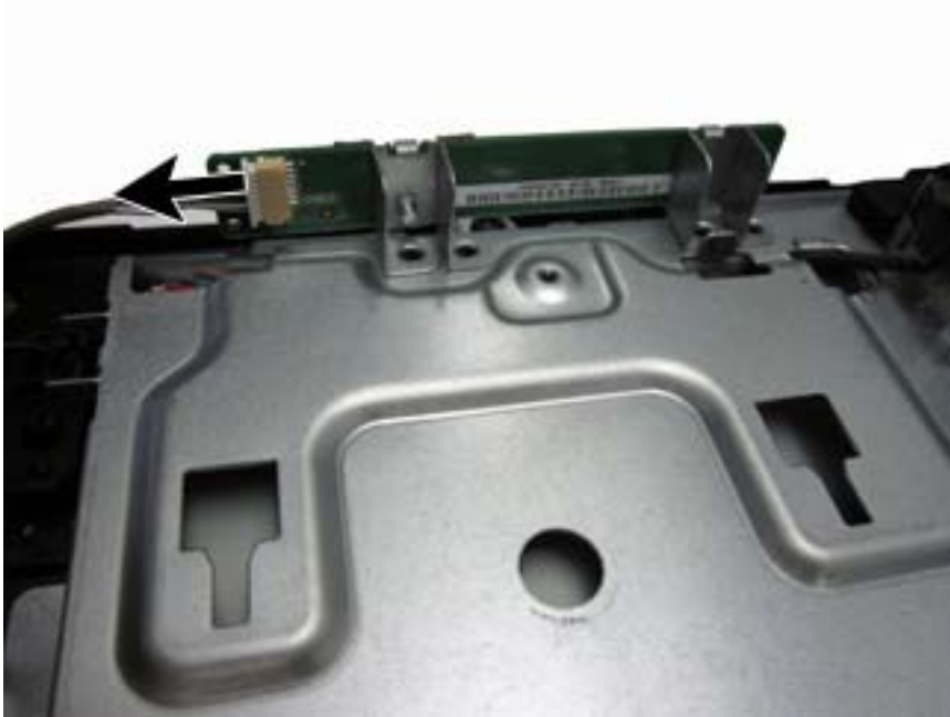
Figure 6-49 Disconnecting the sidekey board cable
