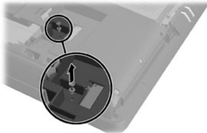
Figure 6-10 Removing the optical disc drive security screw
