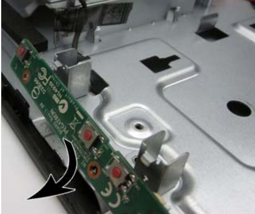
Figure 6-51 Removing the sidekey board
