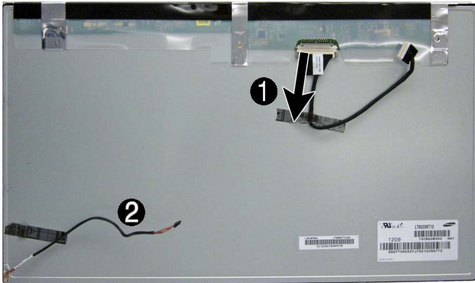
Figure 6-69 Removing the display cable from the display panel
